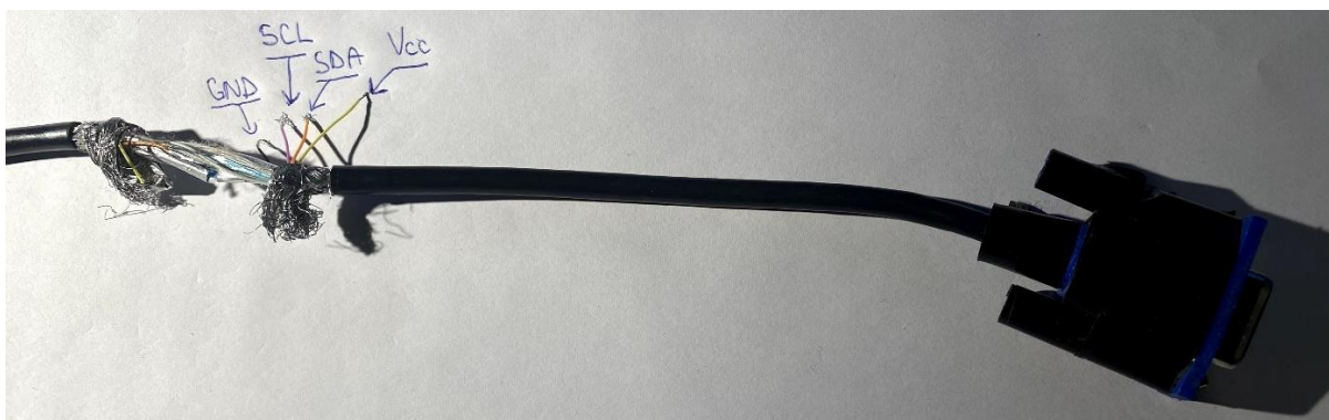
Figure 2. Example of patched VGA cable.
